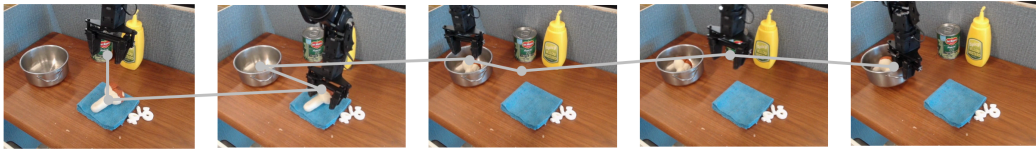
Figure 9: Spatial reasoning failure occurred when masking out low level instruction. The task was to “sweep the mints using the towel.” Due to the presence of the pot and the mushroom, being both strong priors within BridgeData, the policy chose not to follow the high level instruction.
